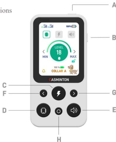
A: ①Long press to turn on/off, ②Double-click to switch back light, day and night mode switch
